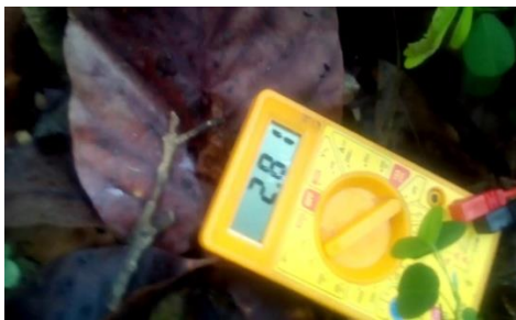
Fig.8.8 Potential difference of 2.81V from Alovera plant
