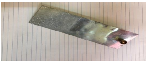
Fig-8.3 Zinc electrode
